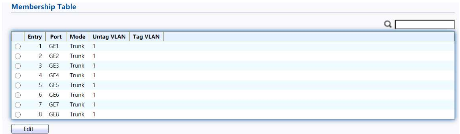
Figure 30 - VLAN > VLAN > Membership
